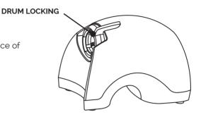
Assemble the feeding entrance and the drum, connect the drum to the main body, and then close the locking device by turning it to 'CLOSE'.
