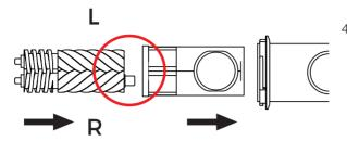
4. With the gear on the right, which has the axis of the Twin Gear, fix it to the drum together with your desired screen.
