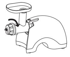
6. When assembling, turn the drum lock clockwise.
